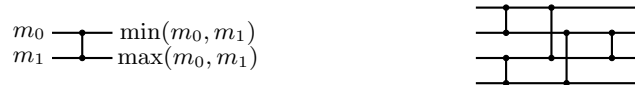
Fig. 1: The basic module and the network of odd-even merge sort for d = 4 .
